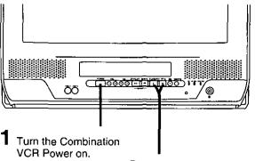
Press and hold both the PLAY and FF on the Combination VCR for more than 5 seconds.
